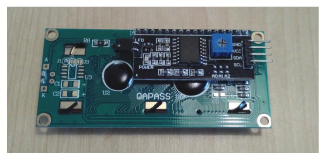
The board on this photo has a PCF8574 port expander chip on it. There are also boards with other chips, e.g. the Adafruit  $I^2$ C/SPI LCD Backpack which uses an MCP23008 port expander.
